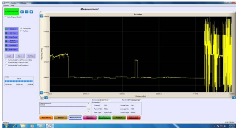
Figure 3. Brillouin Frequency shifts along the fiber, loop back point located at 66.6 km
