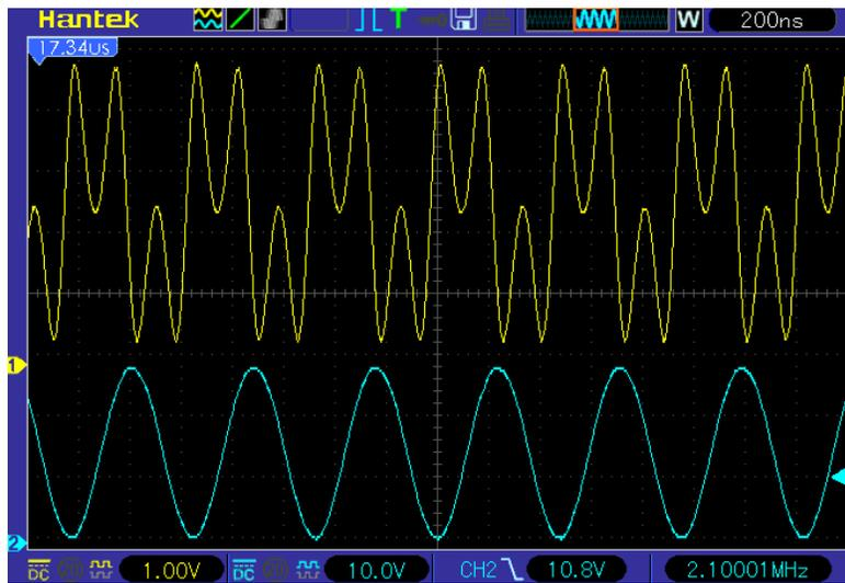
Figure 3. Up to 2.1 MHz modulation rate in  $0\sim 2\pi$  phase shift range.
