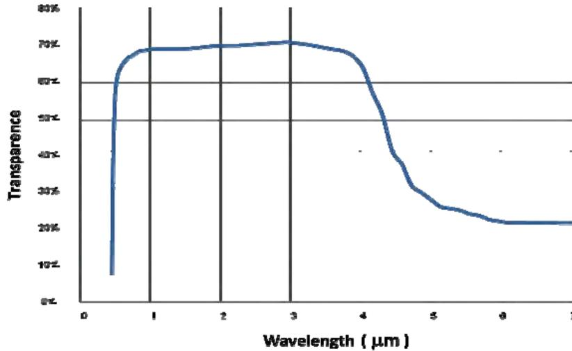
Figure 5. Optical transmission spectrum of EEO crystal wafer with a thickness of 2 mm from 300~7000 nm.
