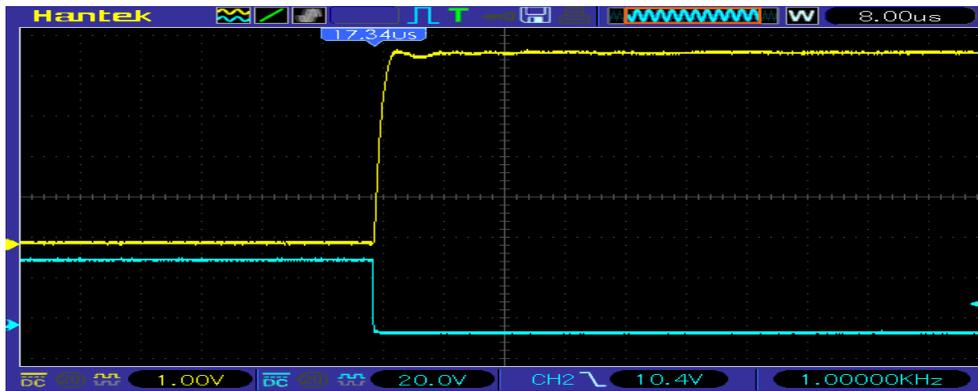
Figure 2. Demonstration of high speed, rising and falling time <math><1.5\mu\text{s}</math>.
