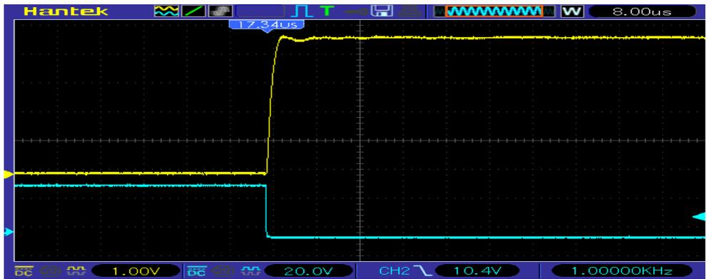
Figure 2. Demonstration of high speed, rising and falling time <math><1.5\mu\text{s}</math>.
