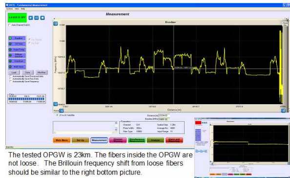
Figure 1: Brillouin frequency shifts along 23-km OPGW.
