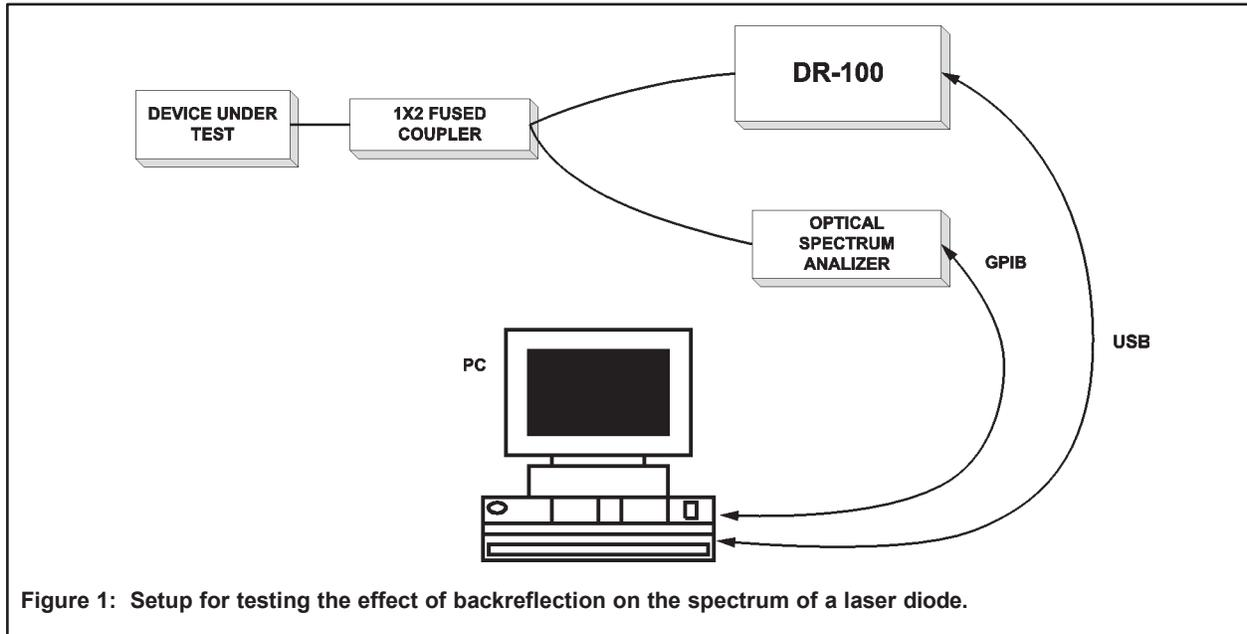
Figure 1: Setup for testing the effect of backreflection on the spectrum of a laser diode.
