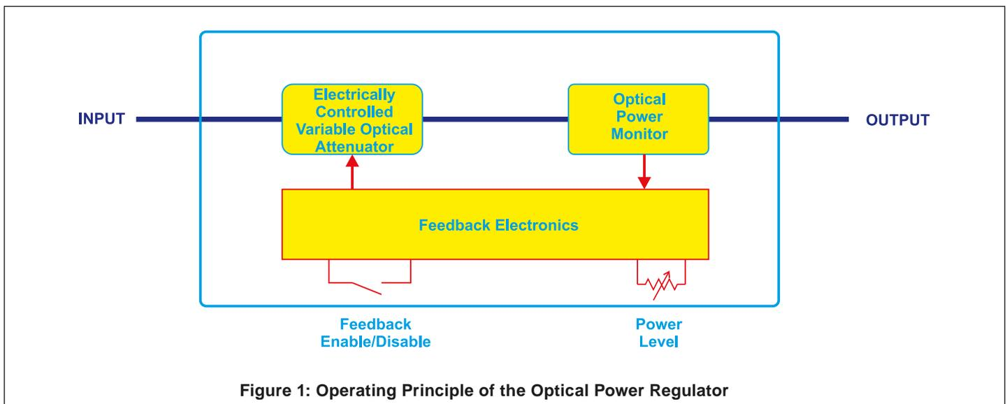
Figure 1: Operating Principle of the Optical Power Regulator
