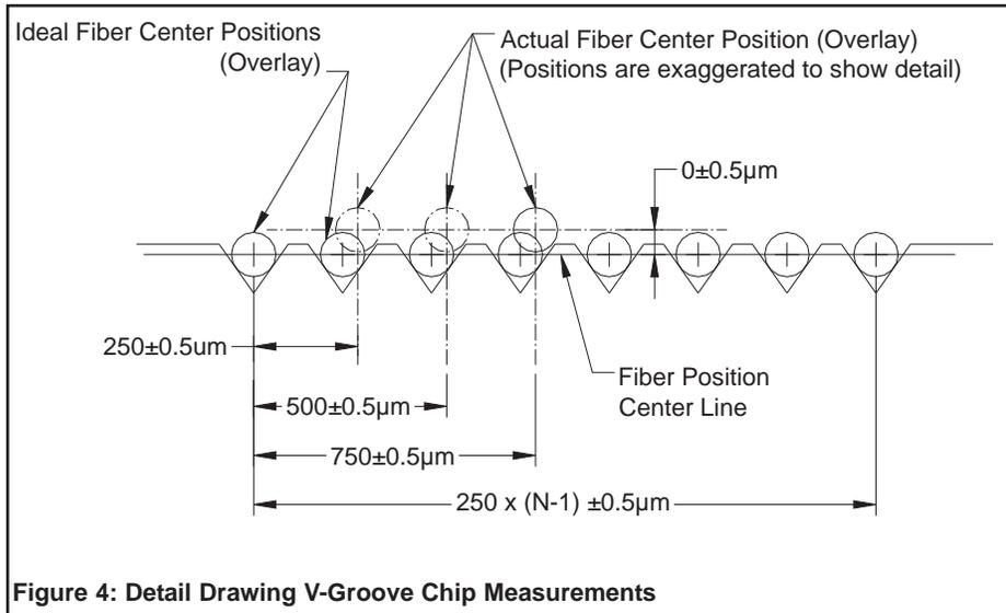
Figure 4: Detail Drawing V-Groove Chip Measurements
