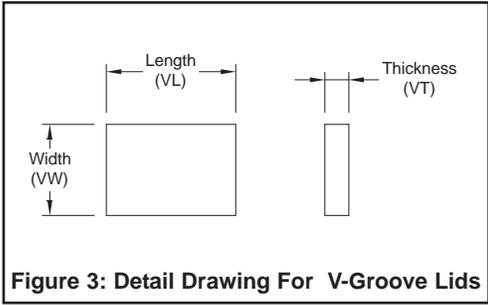
Figure 3: Detail Drawing For V-Groove Lids
