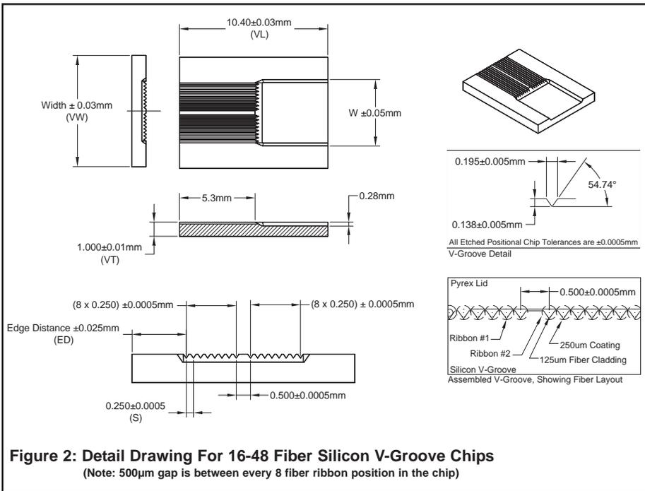
**Figure 2: Detail Drawing For 16-48 Fiber Silicon V-Groove Chips**
