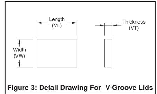
**Figure 3: Detail Drawing For V-Groove Lids**
