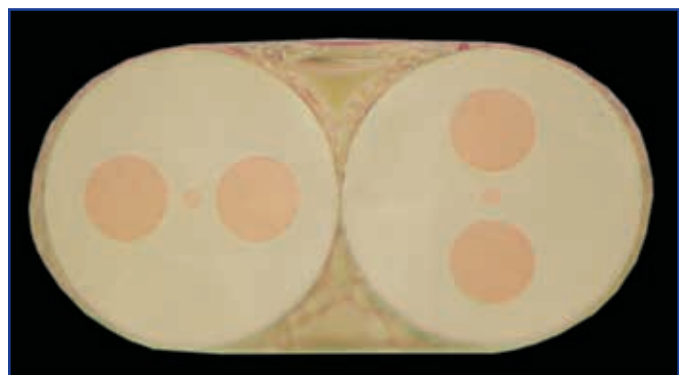
End Face Of Dual Fiber Assembly Showing Stress Rod Alignment
