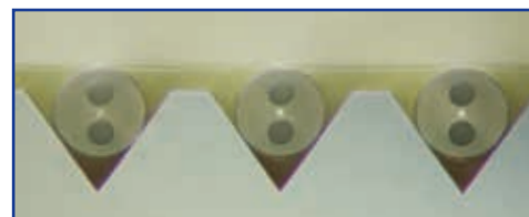
PM Fiber V-Groove Assembly Endface
