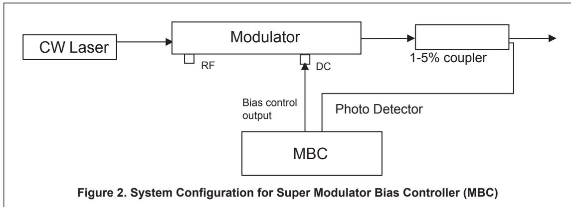
Figure 2. System Configuration for Super Modulator Bias Controller (MBC)
