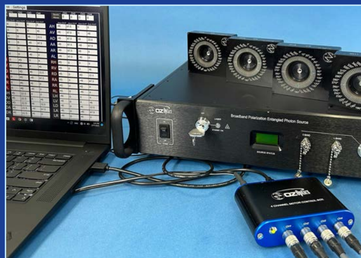
FIG. 1. Quantum Polarization State Analyzer illustrating the two rails of motorized rotation stages and the control unit. In each rail, a rotatable quarter waveplate, half waveplate and fixed polarizer combination allows projection into any single-qubit basis. The two-qubit measurements are then recorded from the two rails feeding two single-photon detectors, connected to a time tagging unit.
